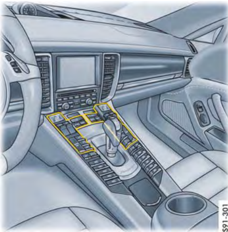
Front air-conditioning control panel
